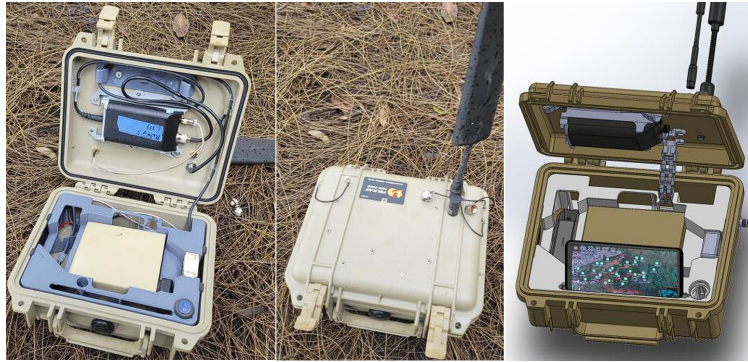
Figure 2: Radio Operations Deployment enclosure seen in-field and in model.
