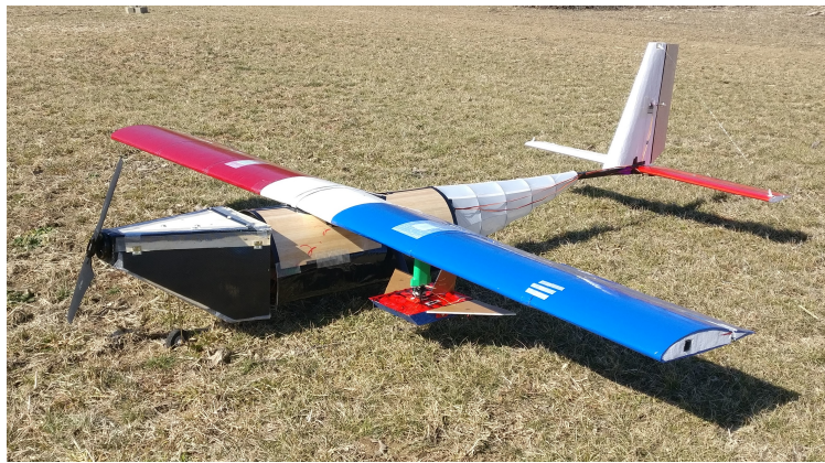
Figure 8: 2020 plane first flight, not the final plane and only including one glider. At competition, there would be two gliders and a slightly resized and more streamline fuselage.
